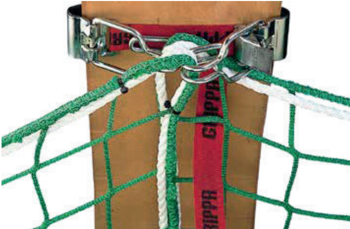
Hanging the edge rope in the hook on the underside of the flange grip in a twisted position prevents unintentional detachment of the net. The two flange grips encircle the I-beam and are closed by pulling a strap with a snap lock.
