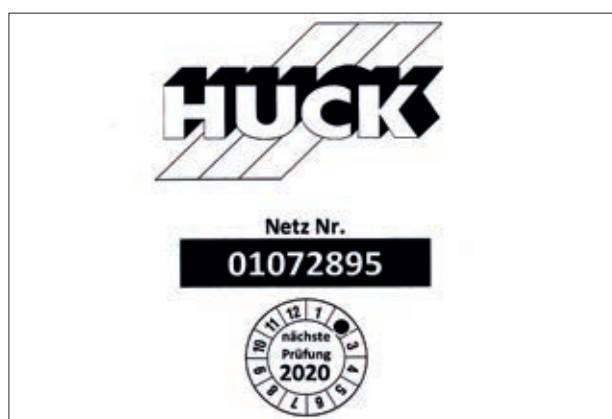
Test badge showing identity number and next inspection date. ④
