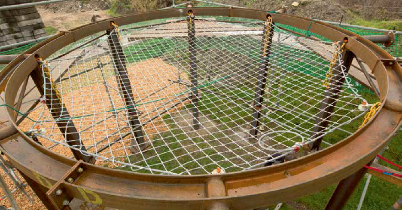
Wire rope net DRALO "XTreme" in test framework.
