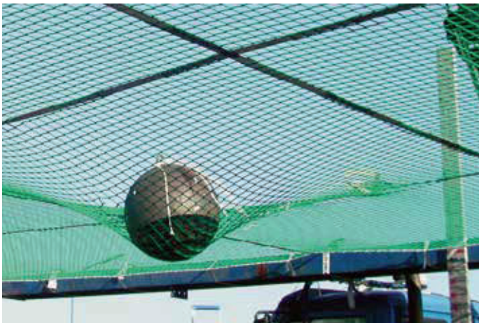
Test: the 100-kg iron ball was dropped onto the net from a height of 3 m.
